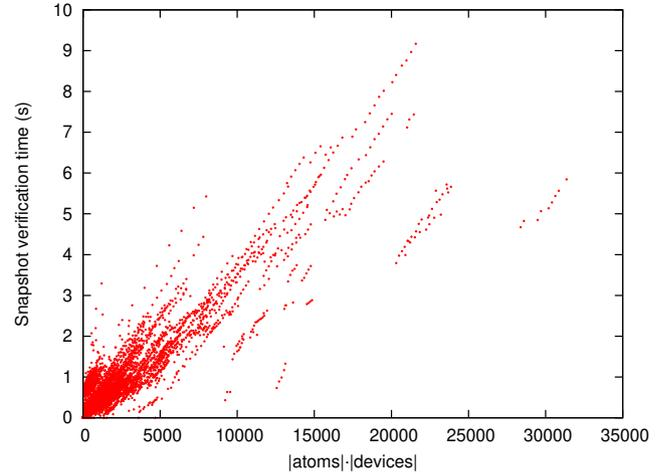
**Fig. 3.** Measured snapshot verification times. Verification time is at most linear in the product of the number of devices and atoms, however it can be significantly lower if many atoms have been added since the last message from collaborating devices.
